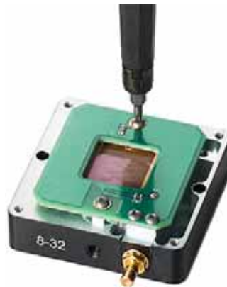
Figure 3-16. Attach Pass-Thru Circuit Board
