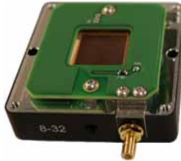
Figure 3-15. Align Pass-Thru Board in Sensor Housing
